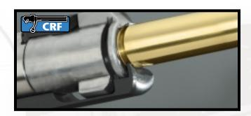
CONTROLLED ROUND FEED BOLT. If there were a single feature responsible for the Model 70 being labeled the "bolt action rifle of the century," it would arguably be the classic, Controlled Round Feed (CRF) bolt design. The massive claw extractor secures approximately ½ of the cartridge base and fully controls the cartridge as it enters the chamber. This unique design also allows the cartridge to be extracted — even if it is not yet fully chambered.
