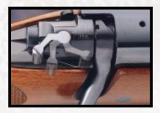
THREE POSITION SAFETY. The three position safety on every Winchester® Model 70 has been proven effective and highly popular by hunters and shooters for over fifty years. Not only is it a convenient reach with the trigger hand, but when the selector is in the middle position you can still operate the action.
