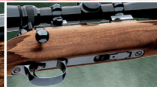
Match grade triggers break clean at 3 – 3.5 pounds out of the box. Receivers bed on twin aluminum pillars permanently bonded into the stock. When it comes to accuracy, there are no shortcuts.
