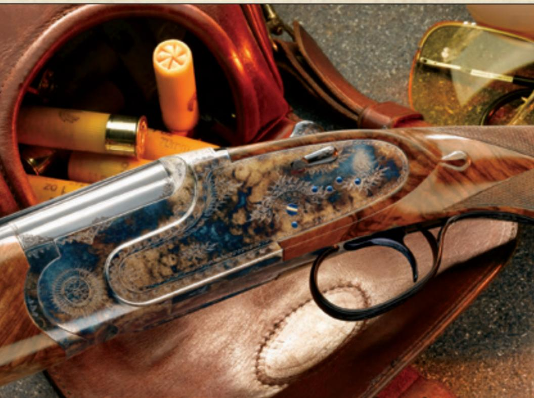
Each Marias shotgun wears scroll hand engraving, bone charcoal case colors and fine finishing touches like niter blued trigger, pins and hammers.
