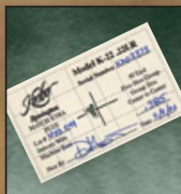
Kimber rifles in .22 LR must shoot a five shot, 50-yard group measuring under .400-inch center-to-center. The test target is included.
