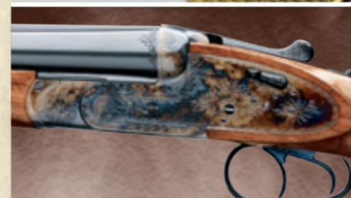
Triggers, pins and hammers wear brilliant niter blue. Locks detach by hand. Barrels have independent cocking indicators. Valier front trigger is articulated
