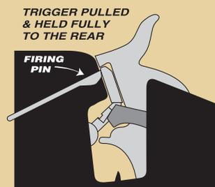
All NEF and H&R single shot firearms incorporate a special safety feature – a transfer bar system that prevents the gun from being fired unless the hammer is fully cocked and the trigger pulled and held completely to the rear.
