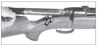
Hold bolt by the bolt handle and extract it from the receiver.
