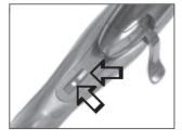
Release safety only shortly before firing the shot. For weapons with set trigger the trigger must be set before firing if it is to be used as set trigger. If the weapon has to be reloaded after firing a shot, the bolt handle must be opened.
