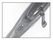
Remove magazine or lock it in second position (magazine protrudes by approx. 5 mm/ 0,19").
