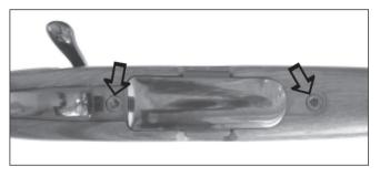
If these screws are loosened, they have to be retightened again with a torque wrench (7 Nm).
