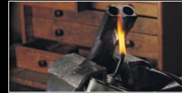
Blacking the breech during jointing
