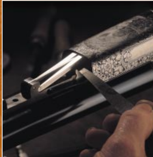
Regulating the Ejector on the Side by Side gun.
