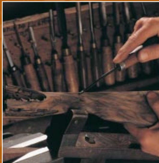
Chequering the hand at 24 lines per inch
