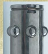
The Heym SR 30 action locking system uses 6 ball bearings that seat in the receiver head. The locking system was tested to 8000 bars (117,600 psi) in a testing series at the proof house in Suhl, Germany.
